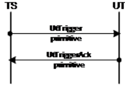
Figure 5: Figure 5.4.4.2.2-1: Trigger message flow
