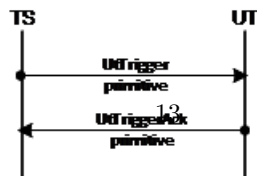
Figure 5: Figure 5.4.4.2.2-1: Trigger message flow
